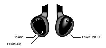
To turn the headphones on and off, push the Power ON/OFF button on the right ear piece. The Power LED on the left ear piece indicates when headphone power is on. Power turns off automatically after 3 minutes of no audio to preserve battery life.
